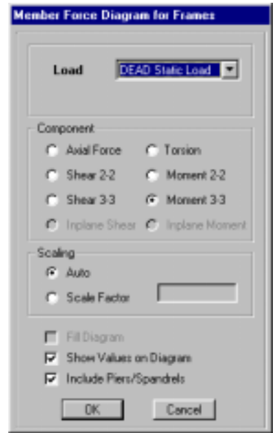
Figure 44 Member Force Diagram for Frames form
